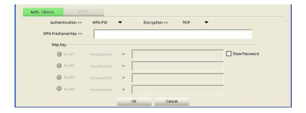
**Step 4.** Please ask the owner of the wireless access point for the security information, and input the correct key here and then click on 'OK'. By checking 'Show Password' box, the encryption key inputted here will be displayed. Authentication type will be selected by the access point automatically, please do not change it.
